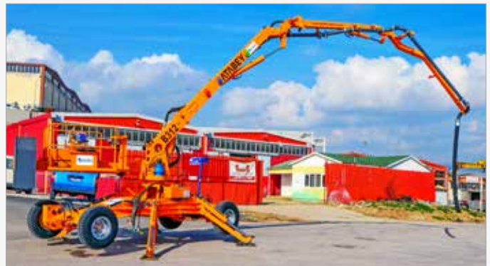
12 meters 4x4 walking hydraulic distributor
